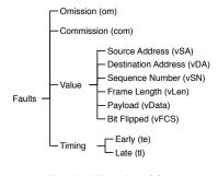
Fig. 4. Hierarchy of faults
