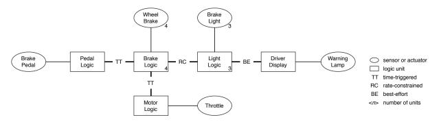
Fig. 5. High-level overview of brake-by-wire system design
