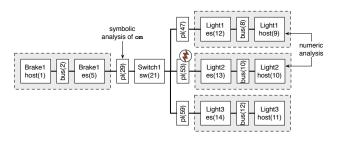
Fig. 10. Example VL 6 (rate-constrained, no path redundancy) with points of symbolic and numeric analysis and fault introduction
